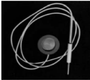
EEG electrode which can be applied to the surface of the skin by an adhesive tape
