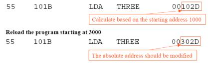
Since assembler will not know actual location where the program will get loaded, it cannot make the necessary changes in the addresses used in the program. However, the assembler can identifies and informs the loader those parts of the program which need modification. An object program that has the information necessary to perform this kind of modification is called the **relocatable program**.
