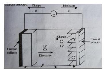
The lithium ion moves from the anode to cathode during discharging and from cathode to anode while charging.
