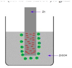
The tendency of the electrode to lose electrons is called oxidation potential and the tendency of the electrode to gain electrons is called reduction potential. This potential difference becomes a constant at equilibrium.
