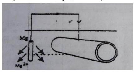
Sacrificial anode systems are based on the position of themetal in the galvanic series. Metals at the top of the series are more prone to corrosion.
