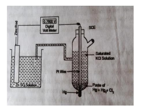
The electrode having higher reduction potential undergoes reduction and is the cathode and the electrode having lower reduction potential undergoes oxidation and is the anode. The reduction potential of SCE is 0.2422V is higher than the standard reduction potential of  $Zn^{2+}/Zn=^{-}0.76$  v . i.e., reduction takes place at SCE and the Zn electrode undergo oxidation.
