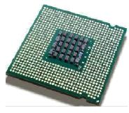
A microprocessor incorporates most or all of the functions of a central processing unit (CPU) on a single integrated circuit (IC).
