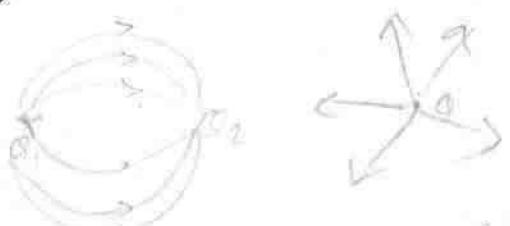
Measure of flow of electric field lines is called flux denoted by  $\Psi$
